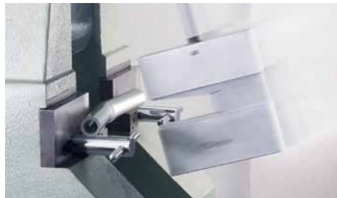
Universal RAUTITAN PN20 pipe tested in the notch impact testing device without breaking at a temperature of -30°C
